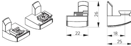
Glass bead support incl. screws for blind type BB24 / BB34 up to a width of max. 128 cm.
