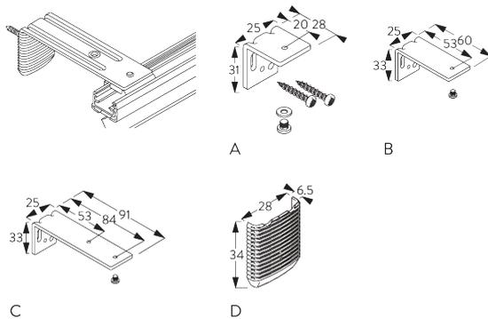
A: Support bracket 28 mm (M1) incl. screws
