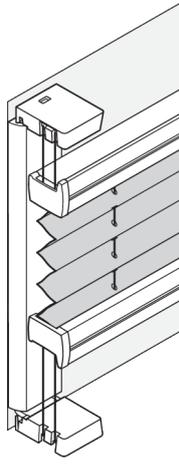
Installation of the system directly on the glass, without any drilling or screwing. The retaining strips are glued to the window pane, then the brackets are attached.
