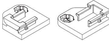
Min. 9 mm straight support surface for blind type BB24 / BB34 up to a width of max. 128 cm.
