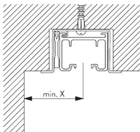
Recess profile SG 2932 can not be bent!
