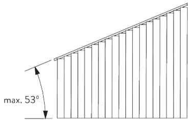
Maximum slope depends on louvre widths:
